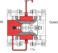
**Tight Closing Operation** Water pressure (equal to inlet pressure) from valve inlet or from upstream of valve is applied to the control chamber. Valve closes bubble tight.
