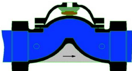
To open the valve, the water or air trapped within the upper chamber is released into atmosphere or into the downstream of the valve, into the pipeline.
