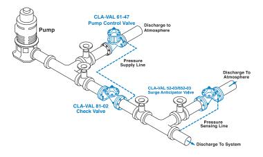
Install Model 61-47 valve as shown. Use a minimum of 1/2" tubing to connect operating pressure connection of the valve to the system side of check valve. Flexible conduit should be used for electrical connections to the solenoid control and the limit switch assembly. A Model 52-02 or 652-03 Surge Anticipator is recommended for power failure and surge protection.
